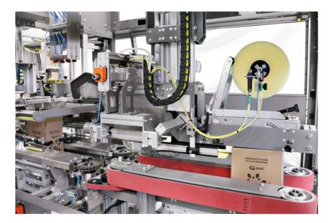
oval containers or briks, simply by changing the gripper / suction cup. This range of machines is particularly suitable for packaging even very delicate and exclusive products such as wines, sparkling wines and liqueurs, without damaging the labels of glass bottles during the packaging process.
