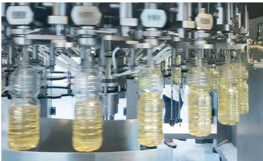
The wide range of solutions offered by SMI also include that with the weight filling system.
