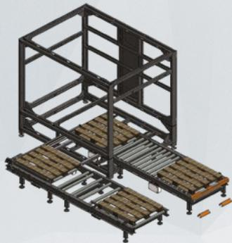
The empty pallet, after having been loaded in the position external to the nets, is automatically brought into the pallet formation area. The pallet 90° transfer is ensured by a pneumatic device (Devio), that, moves the pallet to the desired position thanks to a cylinder. The full pallet is moved to the roller conveyor that is positioned outside the perimeter guards, where it is picked. This solution ensures fast pallet changeover times and minimizes the machine downtime.
