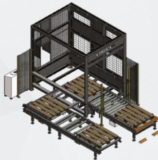
Net guards installed in the machine, except for the pallet loading/unloading area, in which it is instead fixed to the floor. There are a discharge for the passage of the pallet to the empty pallet loading area and light curtains with muting device for the full pallet outfeed area.
