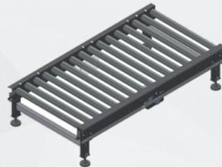
Frame in painted steel and rollers with 76 mm ø 150 mm pitch, motorised through a 5/8 inch chain. Electronically reversible central motorization. The system is tested in SMI factory and is supplied to the client fully assembled and cabled. Available in different lengths: 1500 mm, 2000 mm, 2500 mm and 3000 mm.
