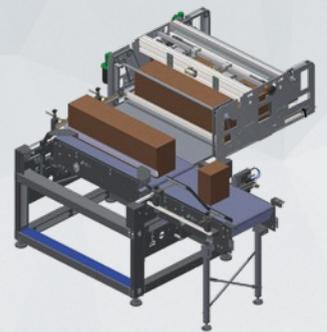
The row transfer process is managed by a motorized bar. After a row is formed, it gets pushed straight away into the loading head (basket). The system is equipped with a "dead" plate (buffer), which enables to continue with the row push-in operations even when the head is not yet in the loading position.
