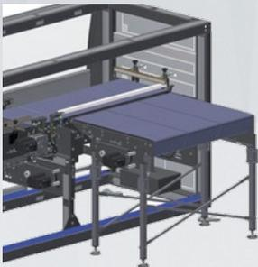
The row transfer process is managed by a motorized bar. After a row is formed, it gets pushed straight away into the loading head (basket). The system is equipped with a "dead" plate (buffer), which enables to continue with the row push-in operations even when the head is not yet in the loading position.
