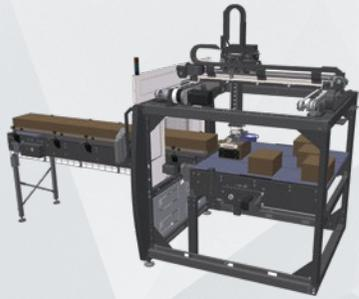
By means of an innovative system of pack rotation and/or manipulation in continuous motion on three Cartesian axes (x, y and z), bundles coming along a belt in single (APS 3070 L) or double (APS 3105 L e 3140 L) lane are turned, shifted and arranged onto
