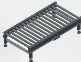
Painted steel frame. Rollers with 76 mm Ø and 150 mm pitch, motorized through a 5/8 inch chain. Electronically reversible central motorization. The system is controlled by the main electrical cabinet. Designed in accordance with FCR (Full Cost Reduction) it is tested and supplied to the customer completely mounted and cabled.
