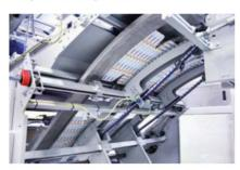
Subsequently, flap-folding devices fold first side flaps and then upper/ lower flaps on both the front and the back of the pack. A gun sprays a thin layer of hotmelt glue on the flaps to ensure a perfect adhesion of the box/ tray.
