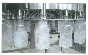
packaging to be managed by a single system, from the preform to the filled, capped and labelled bottle. Also, in the Ecobloc Plus system, bottle movement occurs through direct star-star transfer, allowing for significant savings in terms of initial investment, maintenance costs and energy consumption. The secondary packaging unit, designed by SMI, is an innovative shrink film packaging system.
