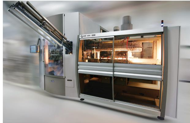
The EBS Ergon series dispenses with cams to minimise energy consumption while maximising performance and ease of use.
